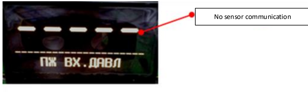
Figure 25. Readings on the display module if loss of sensor connection
